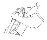
2. Turn the driven clutch moveable sheave clockwise while pushing
